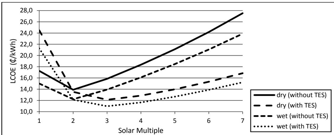
Figure 7. Relation of the Solar Multiple with LCOE to the city of Caicó in the empirical model.
