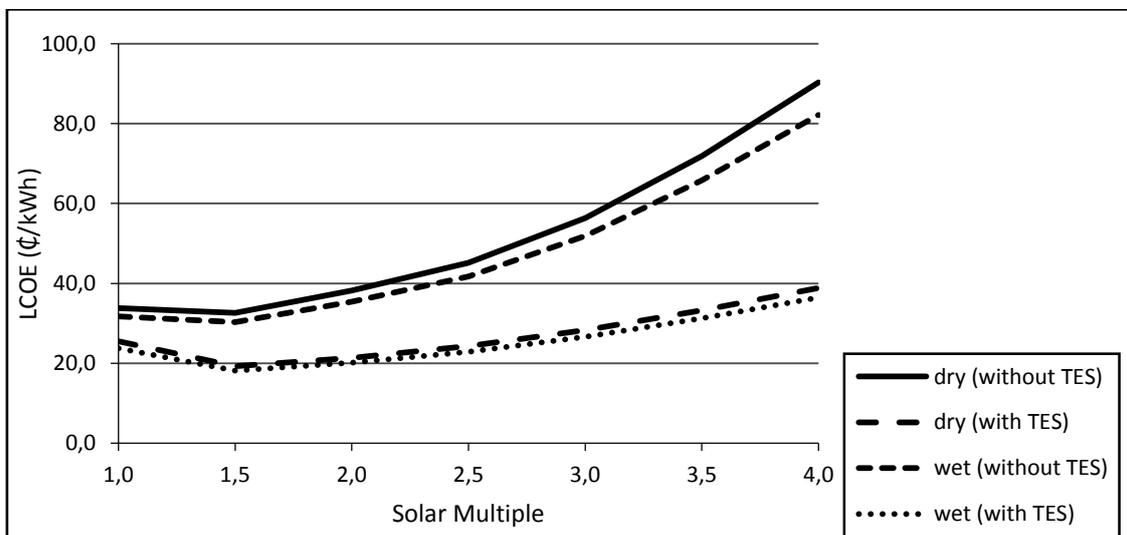
Figure 9. Relation of the Solar Multiple with LCOE to the city of Assú for central receiver.
