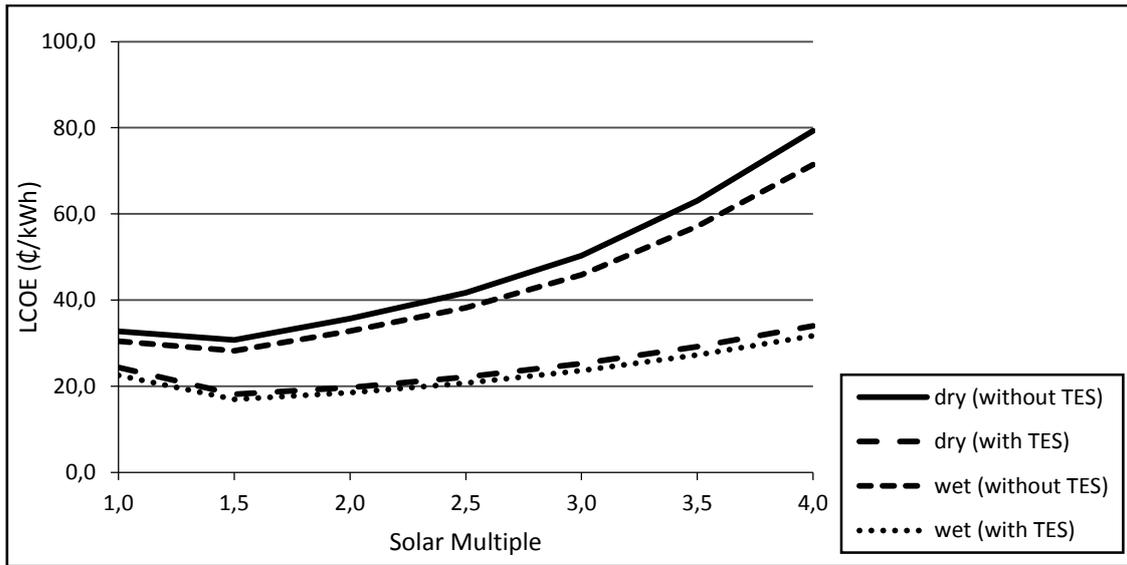
Figure 10. Relation of the Solar Multiple with LCOE to the city of Caicó for central receiver.
