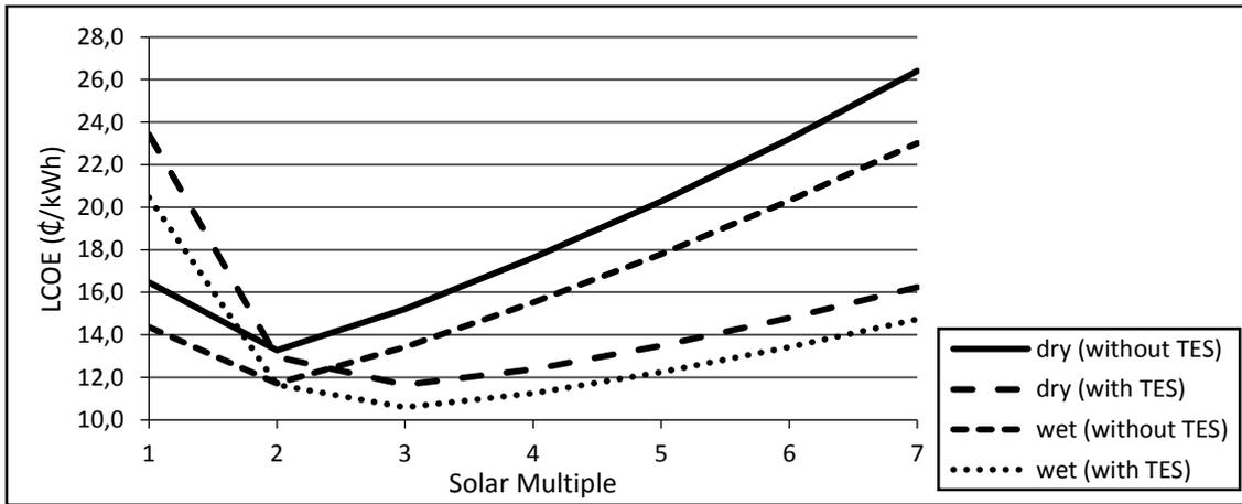
Figure 6. Relation of the Solar Multiple with LCOE to the city of Assú in the empirical model.
