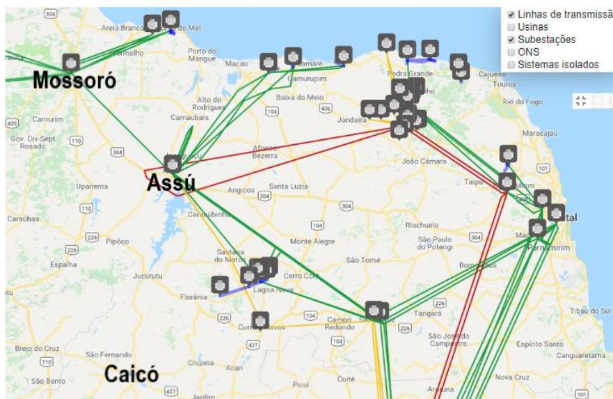
Figure 2. Map of SIN substations and transmission lines in Rio Grande do Norte (ONS, 2018)
