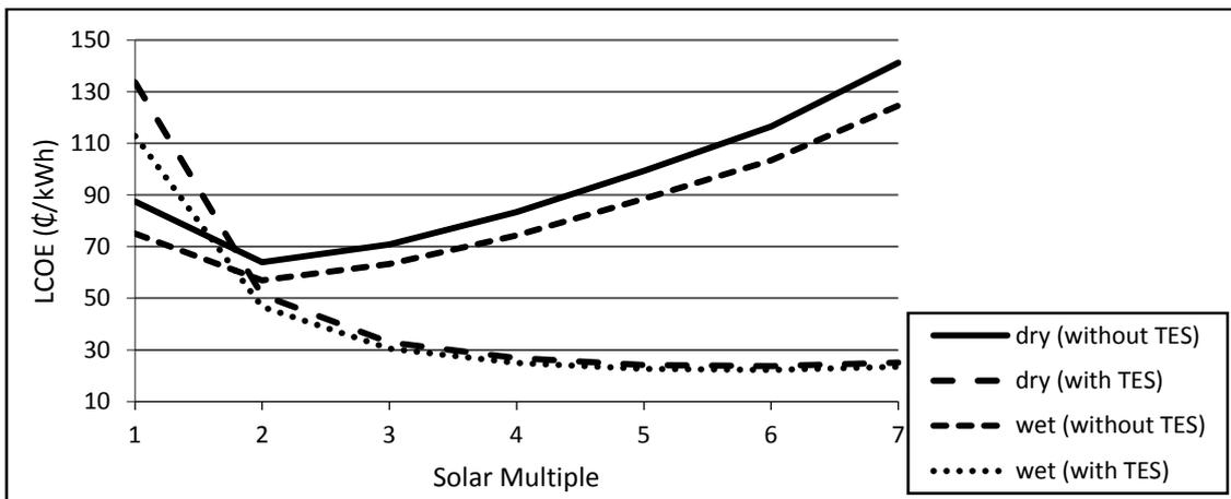
Figure 3. Relation of the Solar Multiple with LCOE to the city of Assú for PTC technology in the physical model.
