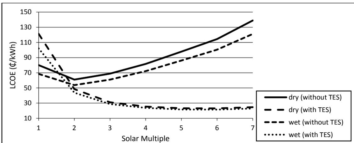
Figure 4. Relation of the Solar Multiple with LCOE to the city of Caicó for PTC technology in the physical model.
