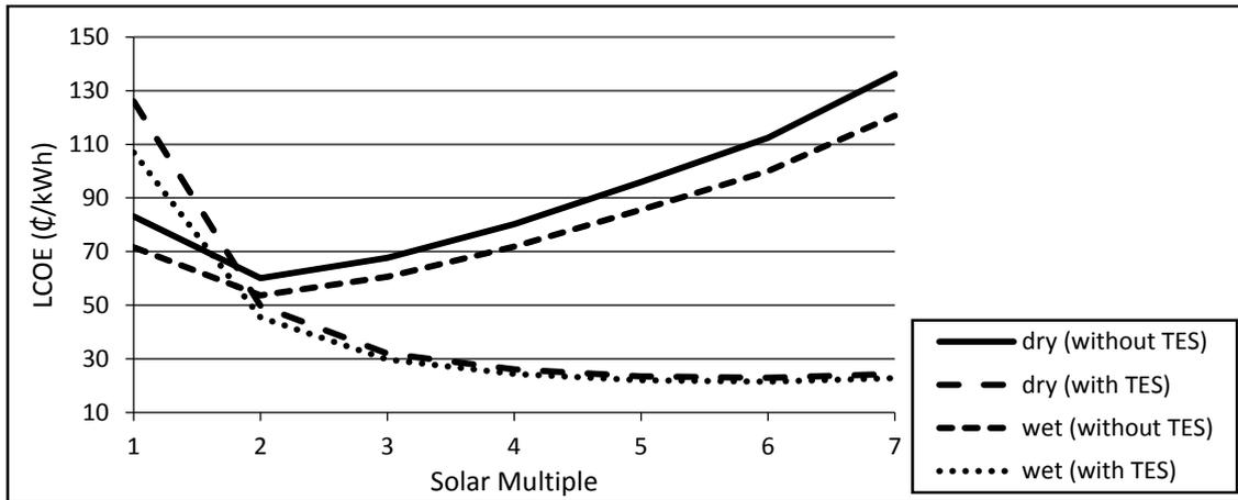
Figure 5. Relation of the Solar Multiple with LCOE to the city of Mossoró for PTC technology in the physical model.
