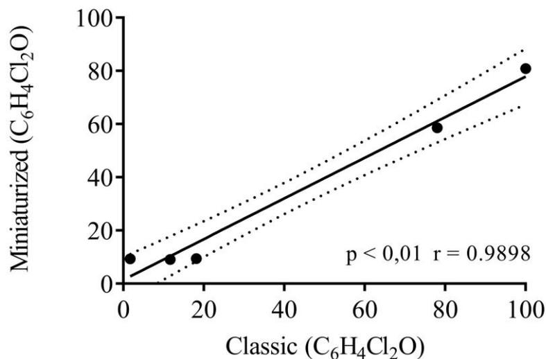
**Figure 1:** Correlation between results from miniaturized and classic test (% inhibition growth of *P. subcapitata*) expose to 3,5-Dichlorophenol ( $p < 0.01$ ;  $r=0.9898$ ;  $r^2=0.9797$ ; 95% confidence bands).
